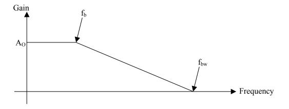
The gain-bandwidth is given at some frequency along the decreasing line. The gain can be found at any point along the line by assuming that the line is a straight line. The y-axis (gain) in this graph is in decibels (dB).  $dB = 20 \log (Gain in V/V)$ . In reverse, Gain in  $V/V = 10^{(dB/20)}$ .
