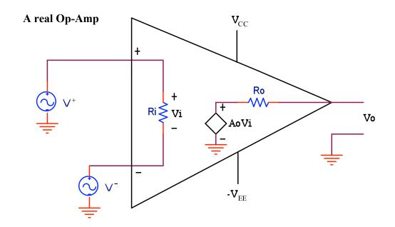
$\begin{array}{lll} \mbox{Ideally:} & \mbox{Reality:} \\ A_O \rightarrow \infty & \mbox{A}_O \mbox{ is less than } \infty \mbox{ and is dependant on frequency.} \\ R_i \rightarrow \infty & \mbox{R}_i \mbox{ ranges from } 2M\Omega \mbox{ to } 1T\Omega \mbox{ } (1x10^{12}\Omega). \\ R_O \rightarrow 0 & \mbox{R}_O \mbox{ ranges from } 10\Omega \mbox{ to } 100\Omega, \mbox{ typically } 75\Omega. \\ \end{array}$
