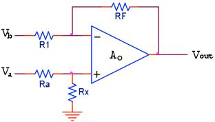
$$V_{out} = -\frac{R_F}{R_1} V_b + \left(1 + \frac{R_F}{R_1}\right) \left(\frac{R_x}{R_x + R_a}\right) V_a \text{ if } R_a = R_1 \text{ and } R_F = R_x \text{ then } V_{out} = (V_a - V_b) \frac{R_F}{R_1}$$
