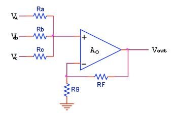
$$V_{out} = \left(1 + \frac{R_F}{R_B}\right) \left(\frac{R_A}{R_a} V_a + \frac{R_A}{R_b} V_b + \frac{R_A}{R_c} V_c\right) \text{ where } R_A = \frac{1}{\frac{1}{R_a} + \frac{1}{R_b} + \frac{1}{R_c}}$$
